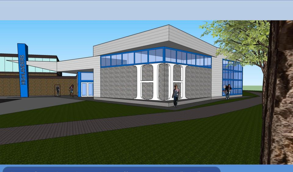
The side facing the parking and drop off area would be a "solid" to address safety issues on approach to the building. To the rear would be full height glass windows allowing views out through the trees.
